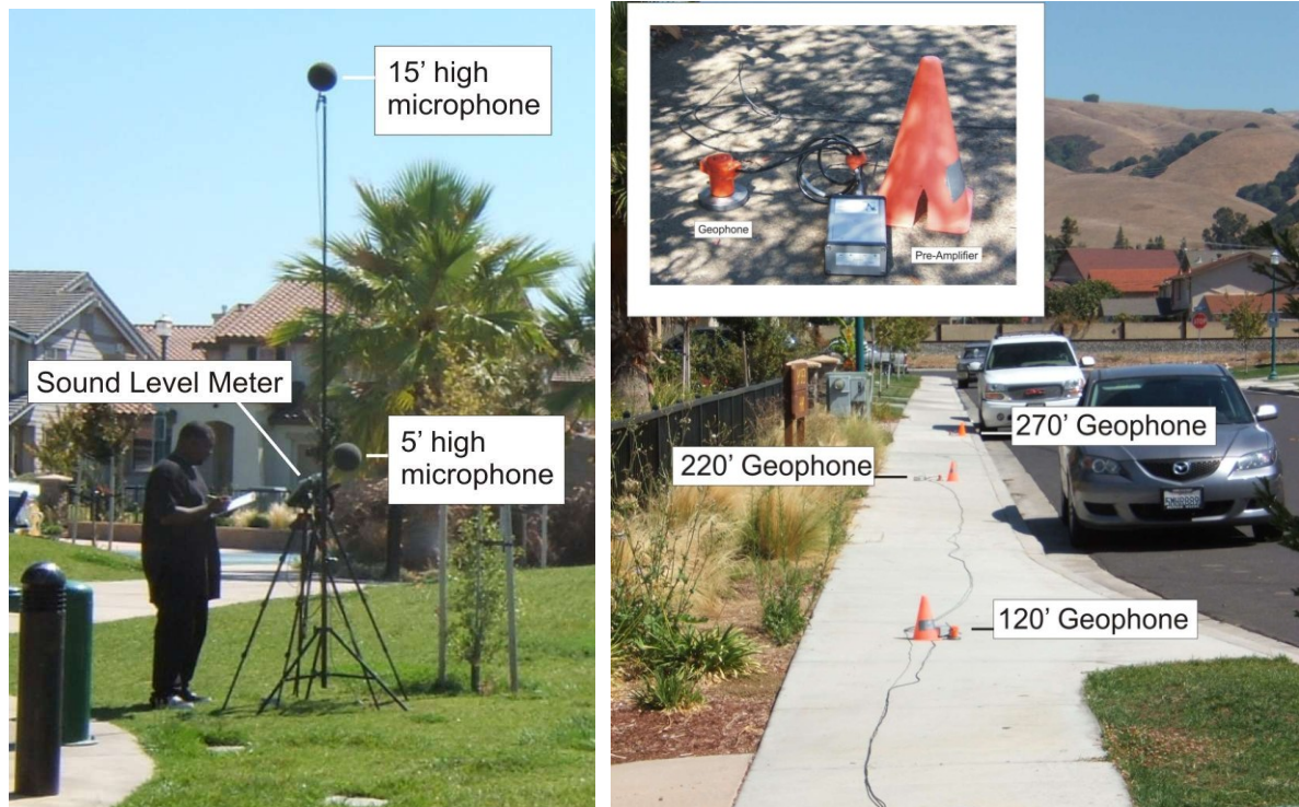
Figure 3 – Equipment setup used for noise and vibration passby measurements
