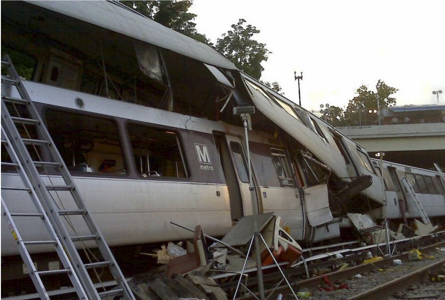
This train collision on Washington, DC's Metrorail system in 2009 was determined to be partially a result of a failed train control system.
