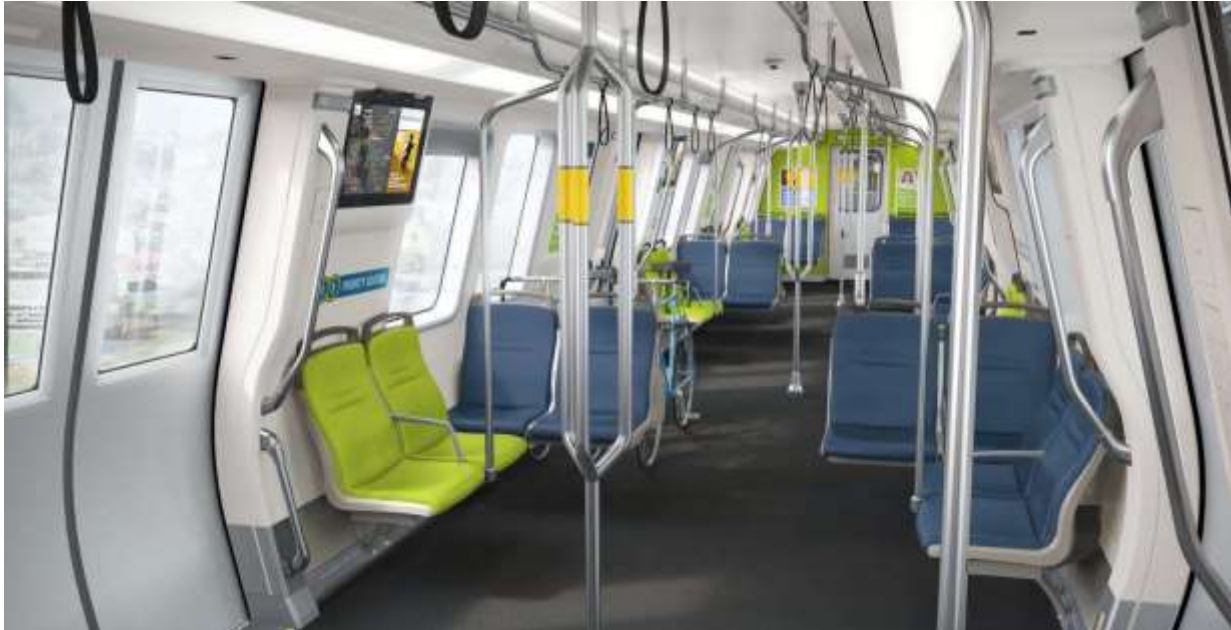
Figure 2-12. Interior of New BART Car, Tripod Poles
