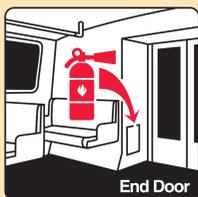
Fire extinguishers are located at each end of car. Kick in plastic door panel to remove.
