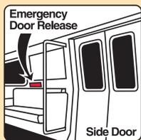
If instructed to open doors in emergency, pull cover panel away and move lever in the direction of the arrow.
