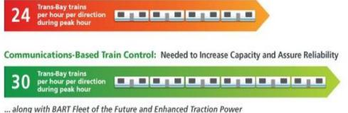
Scope: Upgrade Legacy Train Control System to Communication-Based Train Control (CBTC)
