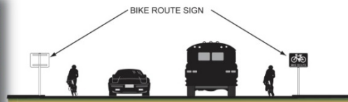
CLASS III BIKEWAY (Bike Route) Provides for shared use with pedestrian or motor vehicle traffic.
