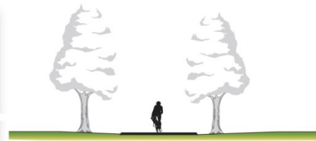
CLASS I BIKEWAY (Bike Path) Provides a completely separated right-of-way for the exclusive use of bicycles and pedestrians with crossflow minimized.
