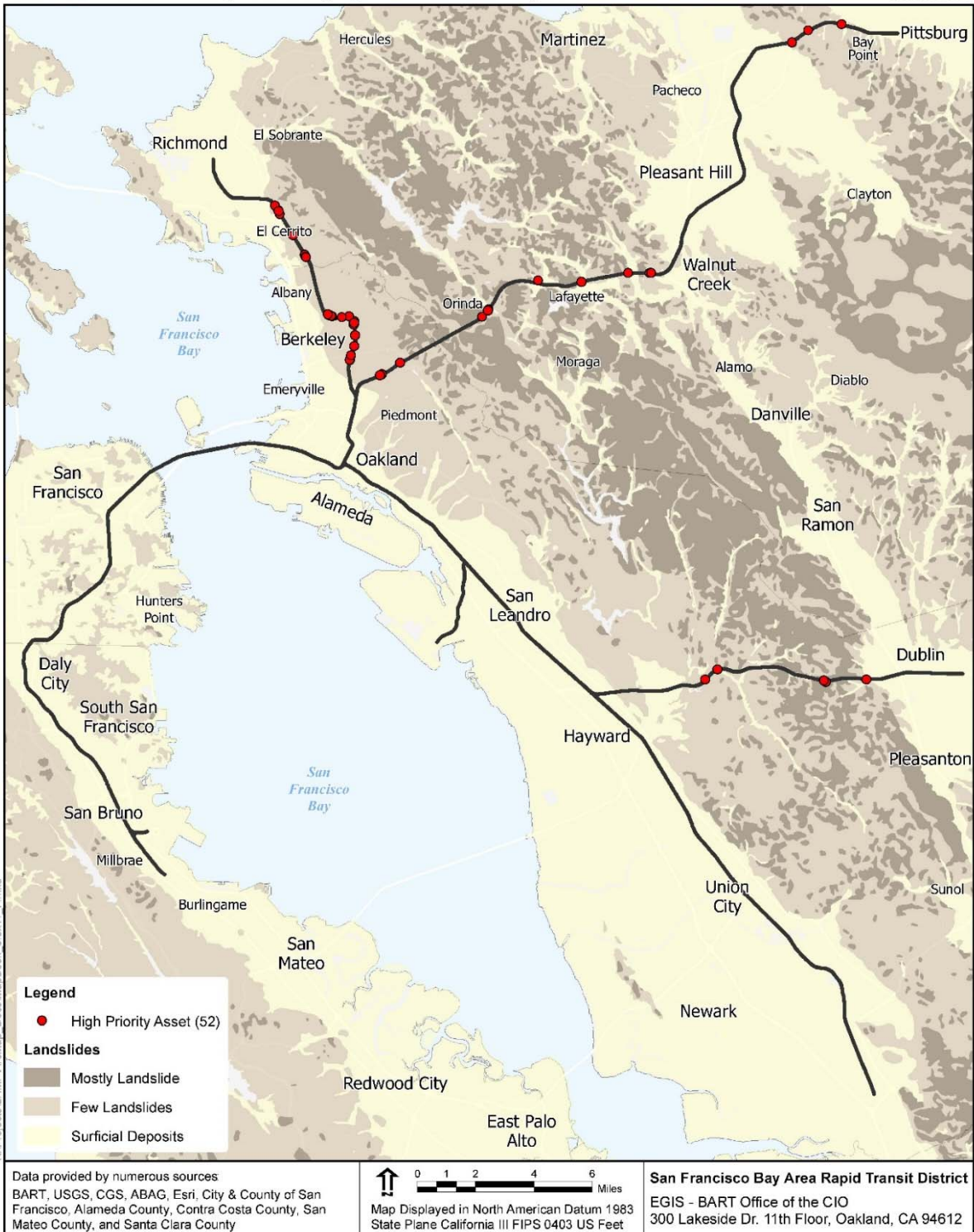
Figure 7 Landslide Zones (Weather)
