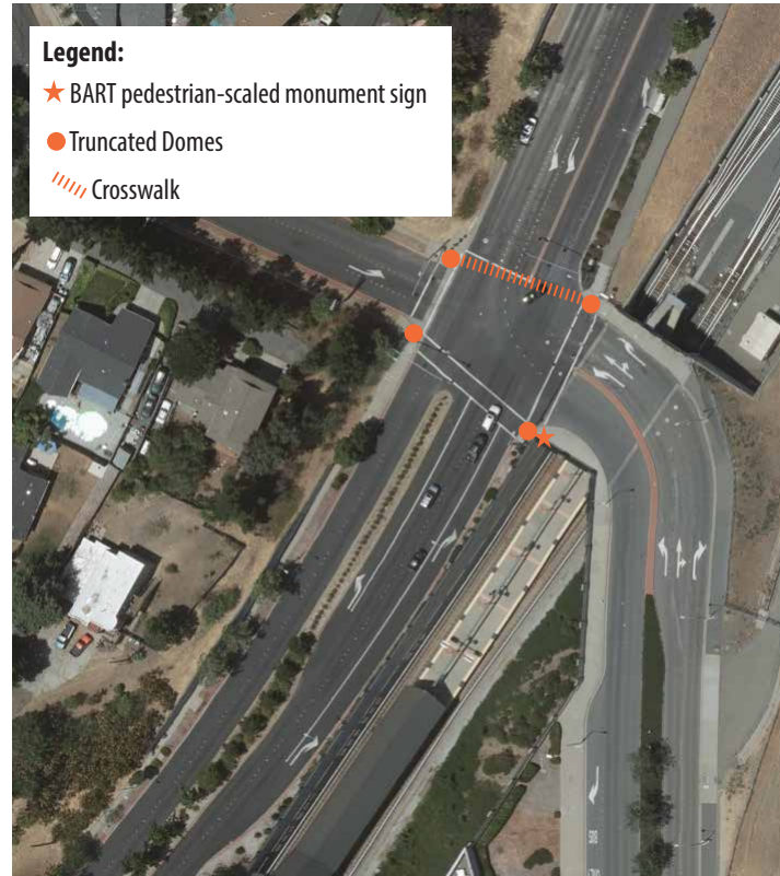
Figure 11 Panoramic Drive Intersection Improvements
