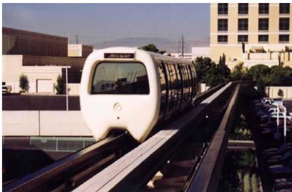
Yantrak Belt-Cable System at Bellagio-Monte Carlo in Las Vegas
