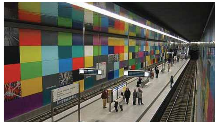
Figure 12: Example of Dual Use Art/Acoustics Tiles
