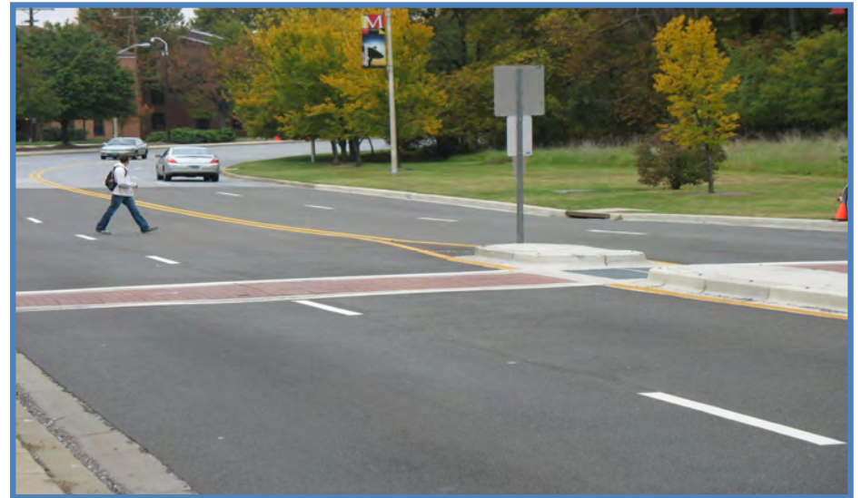
College Park-UMD: Due to bus stop alignment, pedestrians prefer to cross outside the crosswalk
