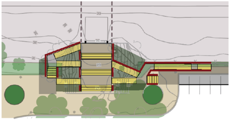
AC-3. RAMP CASCADE PROS: INTEGRATES STAIRS AND RAMPS. LOOKS MORE INTERESTING, PROVIDES MULTIPLE OPTIONS FOR WHERE TO BEGIN. CONS: FULL REPLACEMENT OF THE STAIR AND RAMP FACILITY
