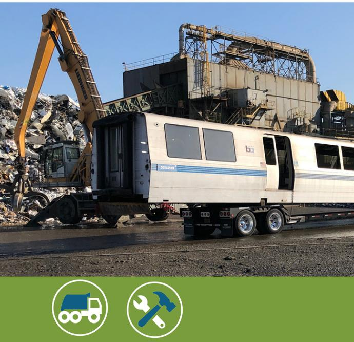
**BART estimates that up to 22 tons of metal is salvaged from each rail car, including 6 tons of aluminum, 1 ton of copper, and 15 tons of steel.**
