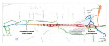
Figure 1. The red oval indicates the location of a Zone 7 pipeline along the south side of 580 between Santa Rita and Isabel Ave.; this could be impacted by the BART project dependent on how far to the south 580 would be widened to accommodate the BART tracks.
