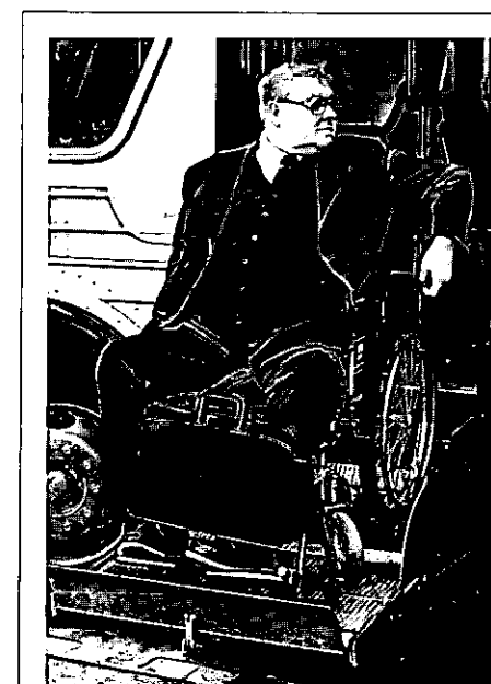
Harold Willson, of Danville, CA, demonstrates operation of the special wheelchair lift on BART Express Buses.
