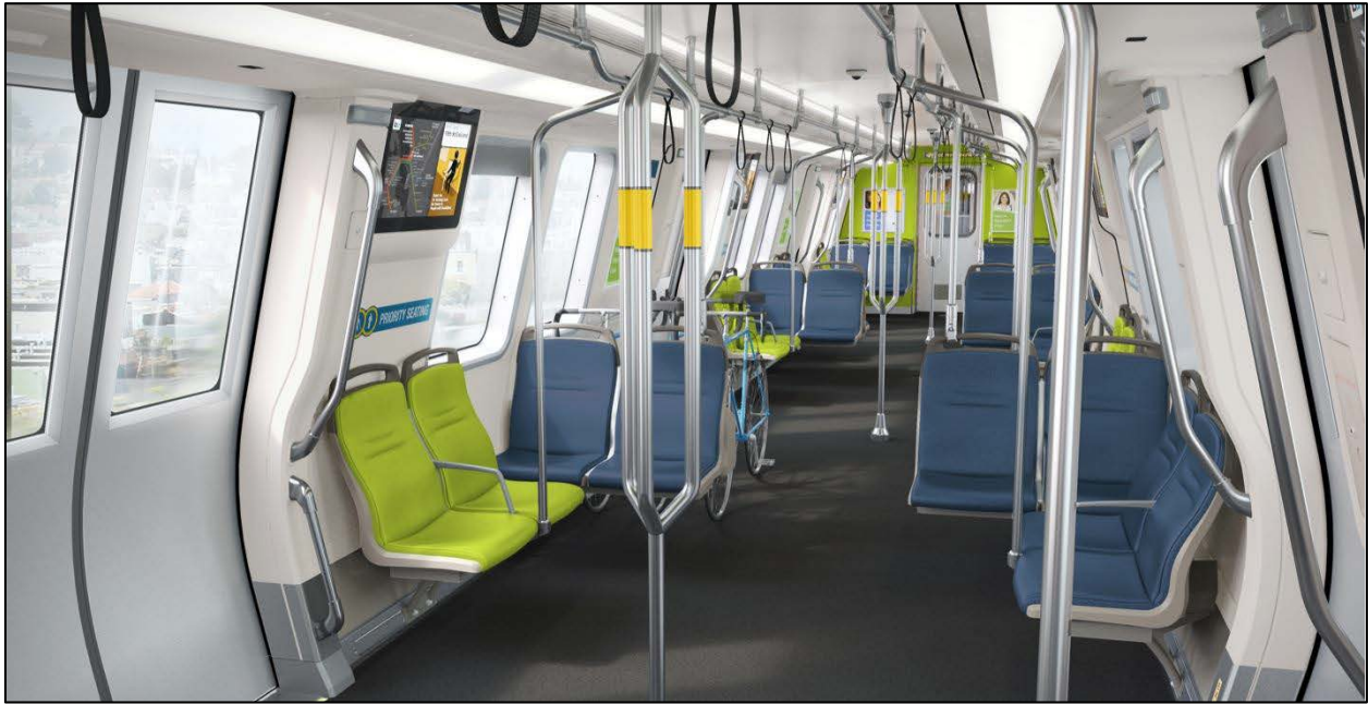
Figure 3. Interior of New BART Car, Tripod Poles
