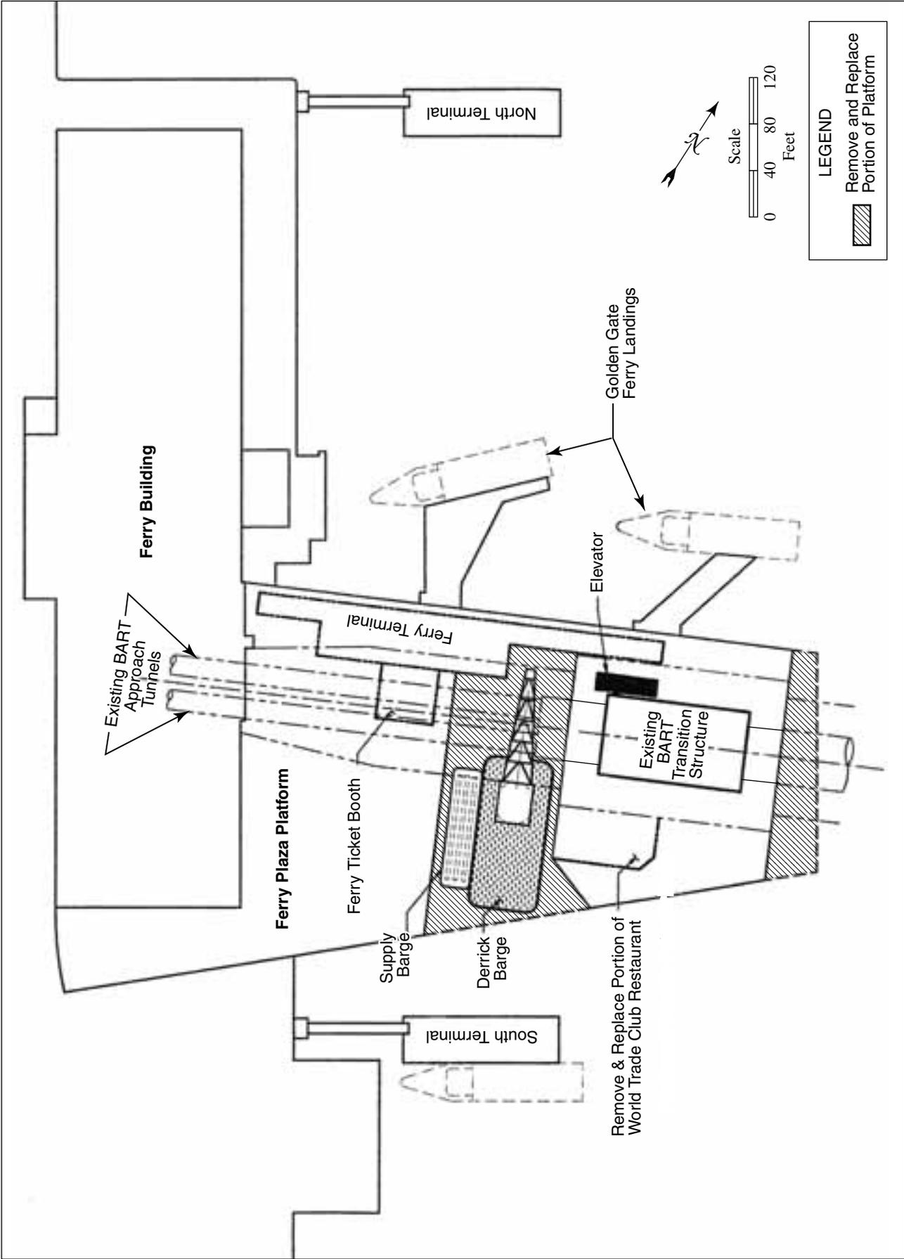
Figure 2-12. Construction Detail for Retrofits at the San Francisco Transition Structure (Construction Method 1)
