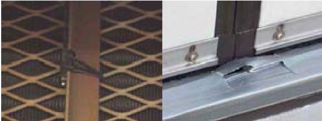
Figure 2-1 ( Left ) Temperature Probe Mounted on Inlet to Condenser Heat Exchanger ( Right ) Temperature Probe Mounted on Car Door to Measure Outdoor Ambient Temperature
