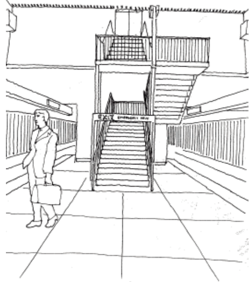
The emergency stair at the north end of the station will be rebuilt to make it wider and less steep.
