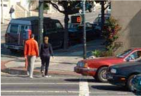
Countdown indicators such as this at Market and Castro streets in San Francisco have cut collisions between vehicles and pedestrians by around two-thirds.
