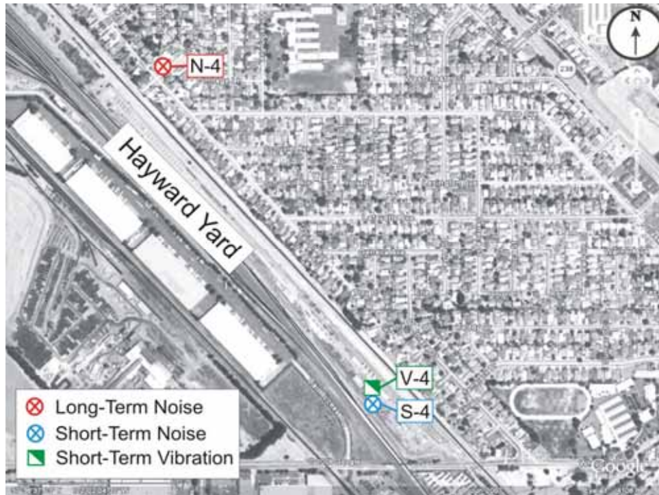
Figure 1 – Long-term and short-term noise and vibration measurement locations (N of Whipple Rd)
