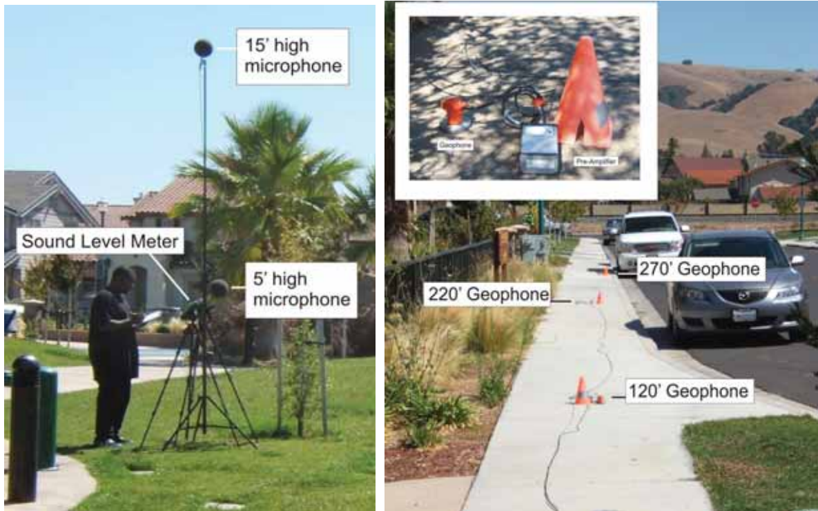
Figure 3 – Equipment setup used for noise and vibration passby measurements
